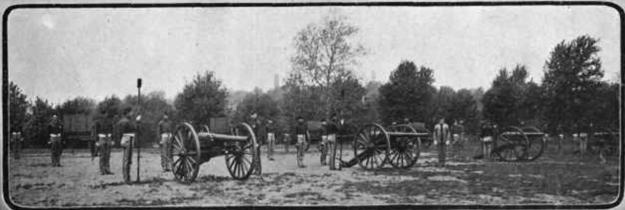
Artillery (four pieces), in action and at rest. The latest pattern 3.2 in., breech loading, steel rifles.
